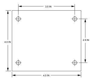
Figure 2: Standoff Hole Placement
